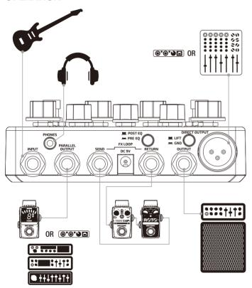
IMPORTANT: TURN ON FIRST, TURN OFF LAST. Always mute the mixer/audio interface or turn down the volume knob on your amp before plugging or unplugging power jacks, cables, etc.
