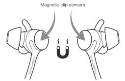
Diagram 4 Magnetic clip sensor location
