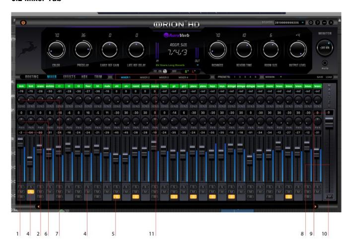
Orion32 HD offers four software low latency mixers which provide zero latency mixing and monitoring that can be distributed to any output from the control panel. The low latency mixers provide all basic functions of a real mixer such as: Solo, Mute, Pan, Stereo Link, Volume Level fader control and a Master Fader - so you can, for example, quickly make a stereo mix plus an Auxiliary send in order to use AuraVerb.
