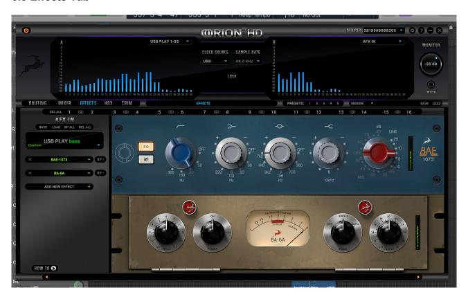
Clicking the Effects tab reveals the 16 AFX Channel Strips. Clicking each bar reveals or hides 2 of the total 16 DSP FX channel strips. Stack effects from the drop-down menu. Drag-and-drop the effects to re-order.
