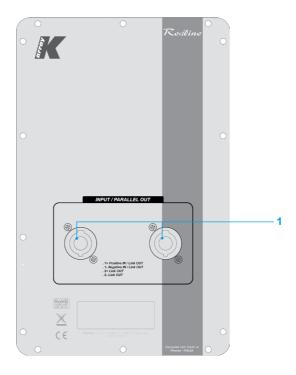
1) INPUT / PARALLEL OUT Speakon connectors. Each connector offers 2 channels of power audio signal. KMT12P and KMT18P internal wiring is designed to pick up audio power signal from pins 1+ / 1- of a NL4 connector. 2+ and 2- pins, just like 1+ and 1-, are directly wired from one socket to the other, so the signal can pass through multiple speaker modules without additional external cabling.
