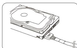
7. Connect "Molex" 4 pin connector, a peripheral device for fans, pumps, legacy components and other devices/adaptors.
