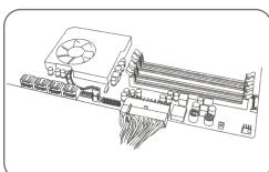
4. Connect the 4 + 4 Pin cable to the main board.
