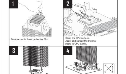
Align the intel cooler base mounting brackets
