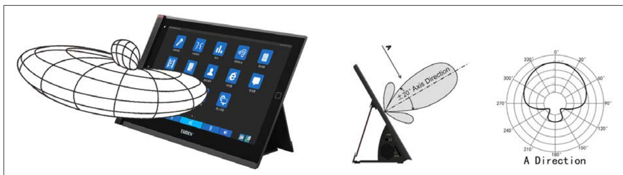
Figure 1.1.9 Polar pattern of HCS-8368A/50 Series G3 Paperless Multimedia Congress Terminal
