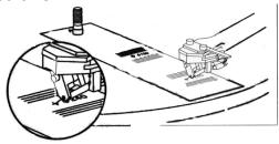
**VTA Adjustment:** The VTA for the installed Goldring Eroica LX cartridge has been properly set at the factory. To adjust the VTA for other cartridges, lay a record on the platter (5). Slacken the horizontal adjustment screws (two **Allen**
