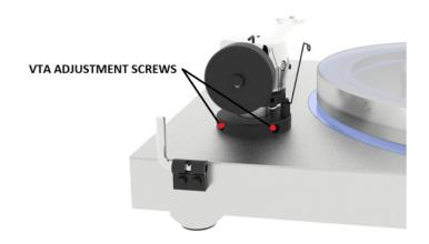
To set the **Vertical Tracking Angle (VTA)**, first put a record (VTF) on the platter. When the needle is lowered into the record groove, the tube of the tonearm should be parallel to the surface of the record. If it is not, loosen both hexagonal screws in the tonearm base, just enough to allow vertical movement of the arm pillar without force, and slide the arm up or down until it is parallel.
