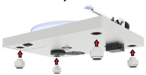
Remove the three feet (5) from the grey foam insert which holds the turntable chassis. Carefully lift the turntable and screw the feet into the thread inserts on the bottom of the turntable. Balance the turntable by using a spirit level before next steps.
