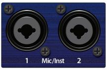
**Microphone/Instrument Inputs.** Both channels of the AudioBox USB96 have Mic/Instrument combo jacks. This convenient connector accepts either a <sup>1</sup>/<sub>4</sub>-inch phone plug or an XLR plug.
