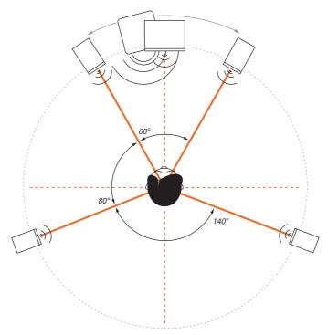
The rear satellites should form an isosceles triangle with the listening position forming an angle of 140°.
