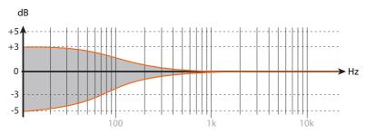
The Low-Shelf Filter allows you to boost or attenuate frequencies below 300 Hz in 0.5 dB steps. Use this filter whenever the acoustics of your room cause problems in the low frequency range.
