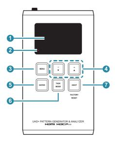
OLED: This screen's layout changes depending on the unit's operational mode and selected function. The status lines at the top shows the unit's current operational mode (Analyzer, Pattern, or Cable Test), USB port mode (power or control), power status, and mode specific detection details. Information below the status lines consists of either the unit's menu or signal analysis data.
