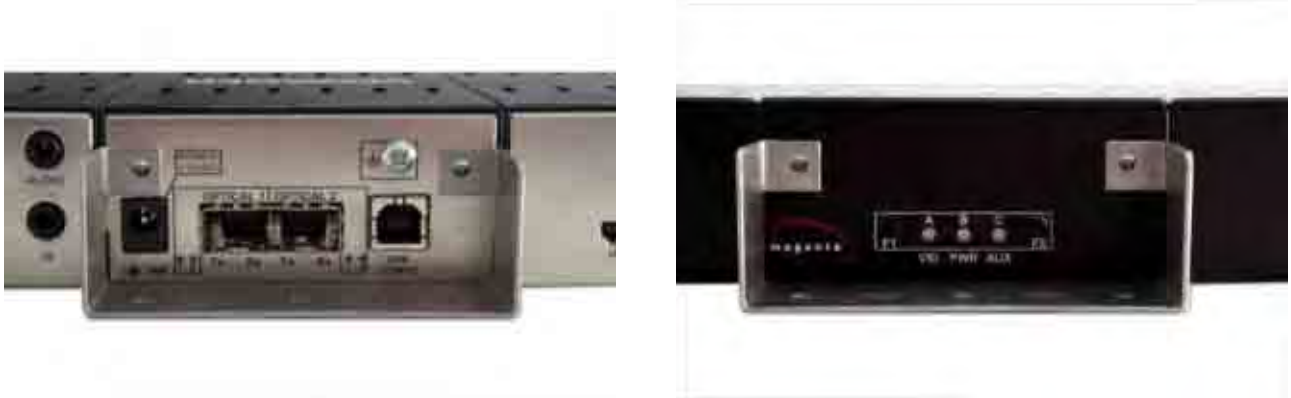
Figure 10. Voyager link Wall-mounting Bracket on rear or front side
