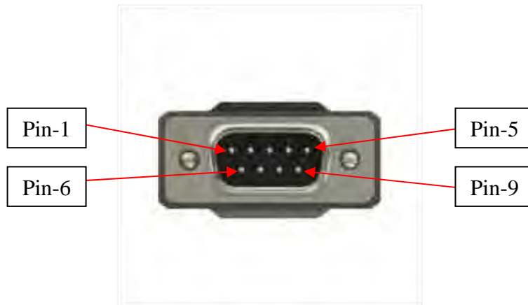
Figure 7. RS232 DB9-Male Pin Numbering
