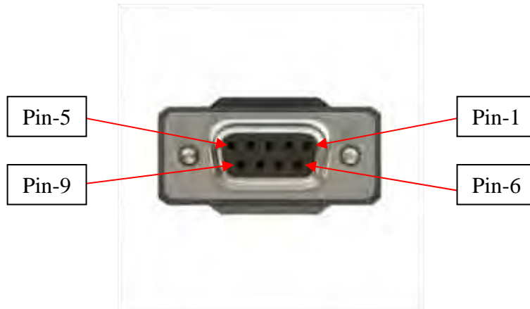
Figure 6. RS232 DB9-Female Pin Numbering
