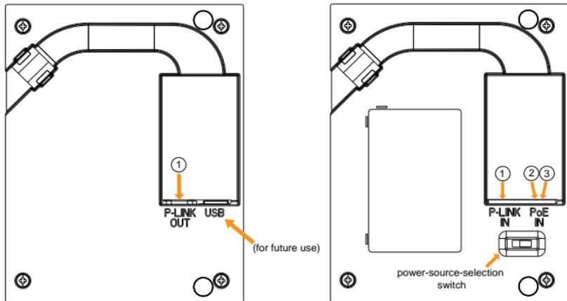
The BFM2 can be powered via a P-Link<sup>1</sup> from CONVERGE Pro 2 (a single cable carries power, audio and control), a PoE power supply<sup>2</sup> (external or ClearOne; a maximum of three BFM2 units can be powered by one ClearOne PoE Injector), or a standard PoE switch<sup>3</sup>.
