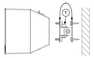
**NOTE:** As a general safety rule, remember to put the runner in place and also that the screw marked "1" should be placed at the upper part of the support, so that if it becomes loose, it will not fall.
