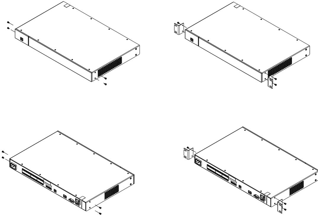
Mount the unit by securing the rack-mount ears to two posts or mounting strips in the rack using the four screws and washers provided. Because the rack-mount ears support the weight of the entire chassis, be sure to use all four screws and washers to fasten the two rack-mount brackets to the rack posts.
