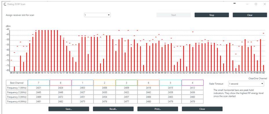
9. Results are shown at the bottom of the screen, with the best channels (those with the strongest signal) ordered from left to right, showing you the best possible channel in your environment:
