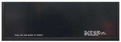
Use these IP addresses to connect to the WebGUI for either the Receiver or Transmitter in a web browser. This will allow for the viewing or control of each unit's configuration and information.
