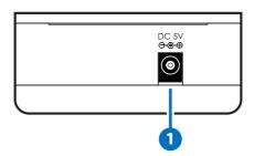
**1 DC 5V:** Connect to the 5V DC power supply into the unit and plug the adaptor to an AC wall outlet.
