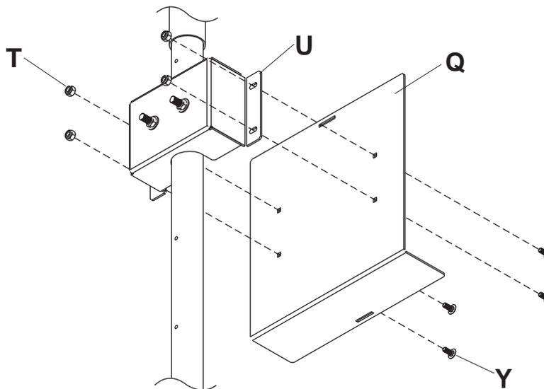
**4** **NOTE:** Use safety belt (Z) instruction in conjunction with this step. Fasten clear strips to the two slots in PC bracket (Q). Set HD box into computer plate (B). Fasten belt with cinch buckle to belt without cinch buckle. Place tri-bar belt clips and belt guide onto belt as shown in the safety belt instructions. Feed the ends of the belt through the PC bracket (Q) slots and through tri-bar belt clip. Cinch the end of the belt so that the PC is securely held.
