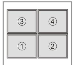
**Note:** Install/adjust the displays by the numerical order given.
