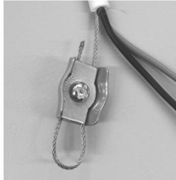
5. In order to make the installation totally secure, introduce safety cable in the eye bolt too.
