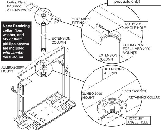
Thread extension column into threaded fitting in ceiling plate. Tighten securely - four or five complete turns. Align slot with one hole in side of threaded fitting. Lock extension column with one M5 x 10mm phillips screw.
