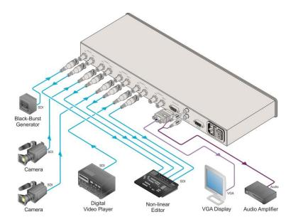
Figure 3: Connecting to the SP-4D Rear Panel
