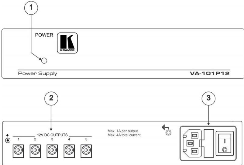
Figure 1: VA-101P12 5-Output 12V DC Power Supply
