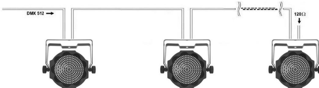
Use a cable conforming to specifications EIA RS-485: pole twisted, shielded, 120Ohm characteristic impedance and low capacity (PROEL DMXD – DMXD1).
