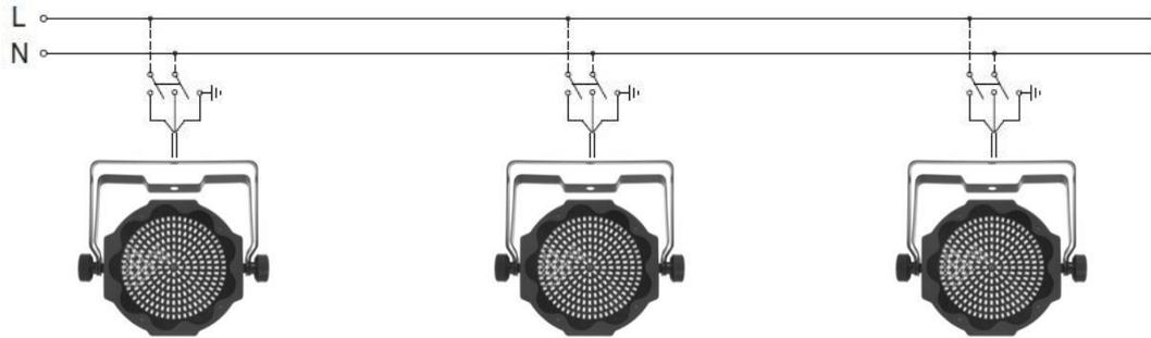
The device must be connected to a power supply system with a proper earth system. Moreover, it is recommended to protect power supply lines of the products from indirect contact and / or shorting to earth by using appropriately sized anti electrical shock switch. The electrical connection must be carried out by a qualified electrician. Ensure that the mains frequency and voltage correspond to those for which the device is designed, as shown in the electrical data label.
