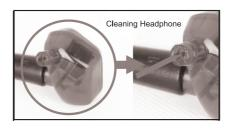
If you notice a change in sound quality, remove the sleeve and check the nozzle of your headphone. If nozzle is blocked, using the cleaning tools to clean the nozzle, such as toothpick.
