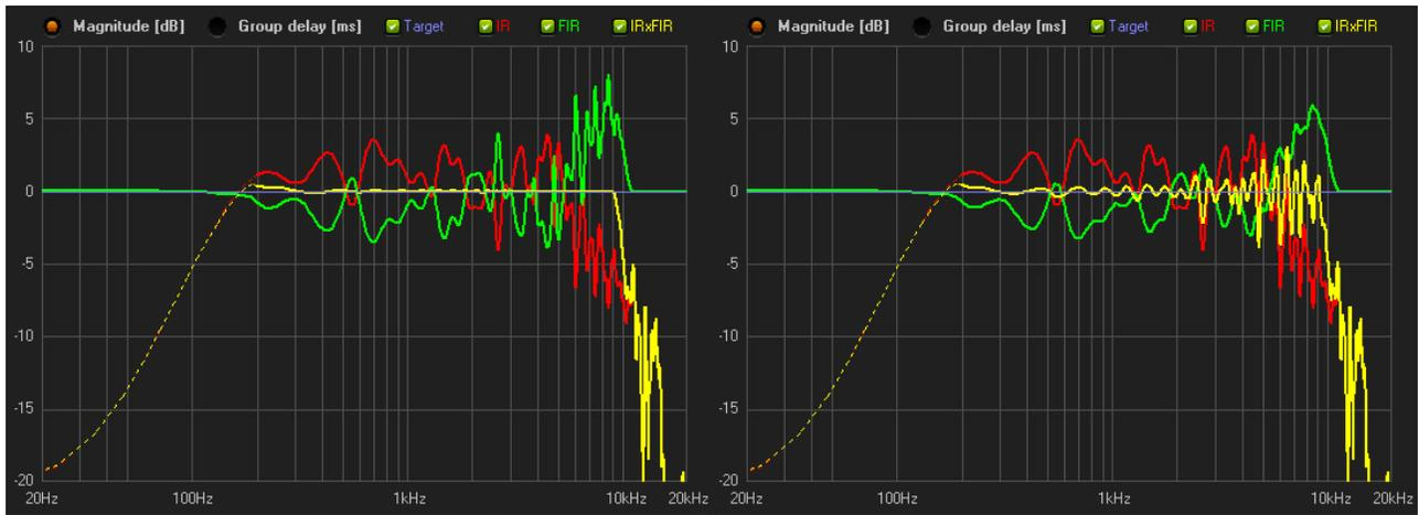
When the “Magn+Phase” mode is selected, the phase smoothing is always applied to the whole frequency range, even if the threshold is not equal to 0dB.
