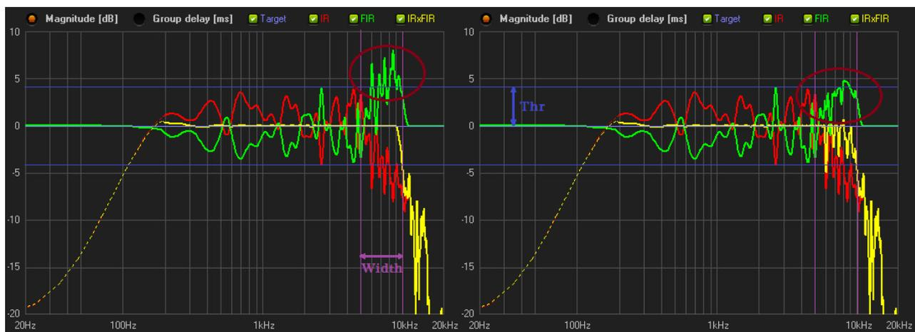
Setting up the threshold to 0dB, the smoothing is applied to the whole magnitude response, as shown in the following picture (left side plot, smoothing disabled; right side plot, smoothing enabled)
