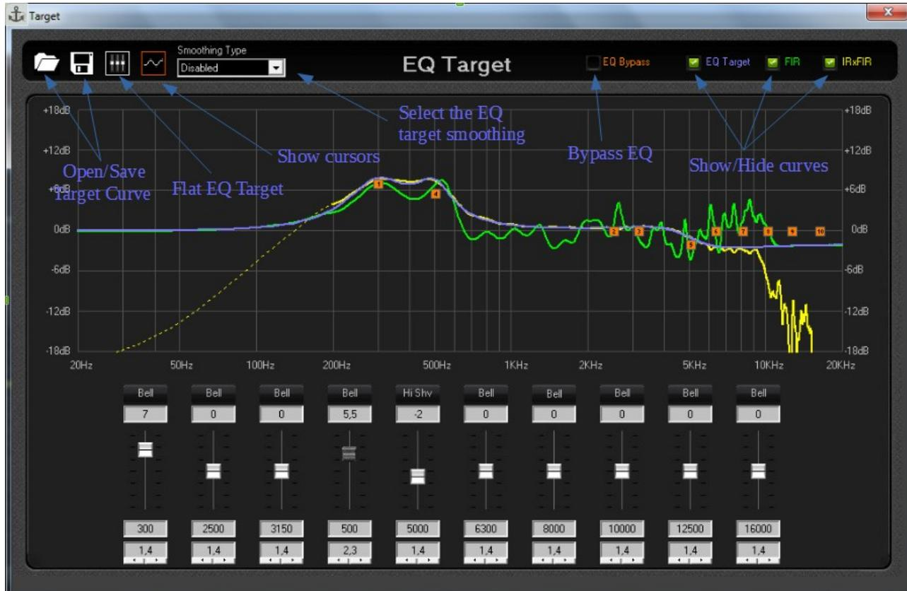
The EQ target can be bypassed (or enabled) by clicking the “EQ Bypass” checkbox at the top center of the screen. Clicking the “Flat EQ Target” button, the gain of each parametric filter is set to 0dB to flatten the target curve.
