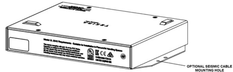
Figure 5 TCM-X Seismic Cable Mounting
