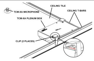
Figure 8 Above-Ceiling Tile Corner Installation Option
