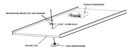
Figure 4 Above-Ceiling Tile Installation Option
