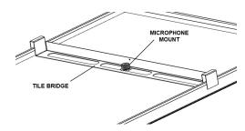
Figure 6 Above-Ceiling Tile Bridge Installation Option
