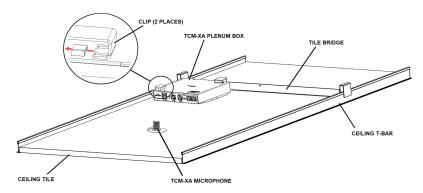
Figure 7 Above-Ceiling Corner Tile Bridge Installation Option
