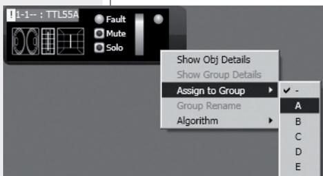
Right-click again the object and now choose 'Show Group Details' to open the common equalization window (settings can be made in the same way as a single object as long as assigned to a group).
