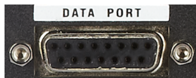
Figure 2.12: I 2 C Data Port
