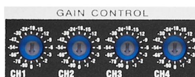
Figure 2.6: Digital Level Controls (endless)
