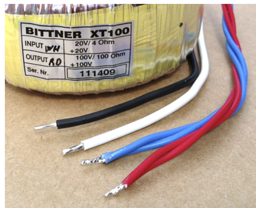
Figure 3.35: XT Transformer - Connection Wires and Sticker
