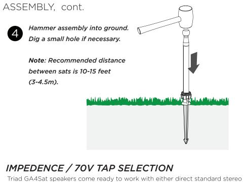
amplifiers or 70/100V systems. Comfirm that the dial underneath the enclosure is set to the appropriate value for your amplifier and number of connected speakers. The total wattage of all speakers should equal 80% of the amp's maximum output. For the Crown CDi 600 amp, the total watts should be 480 per channel. Appropriate combinations would be 16 GA4 Sats set to 30 watts (16x30=480), 32 GA4 Sats set to 15 watts (32x15=480), etc.
