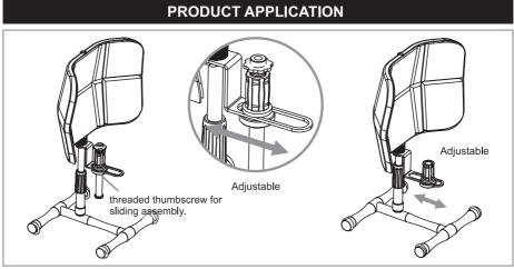
Loosen the threaded thumbscrew for sliding assembly(E), you can horizontal adjust the position of microphone through extension bar. Until microphone in the proper position, then you can fix the threaded thumbscrew for sliding assembly.
