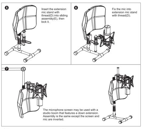
NOTE: when extension mic stand with thread(D) is in the highest position or down extension, use jacking block(G) to lock it.
