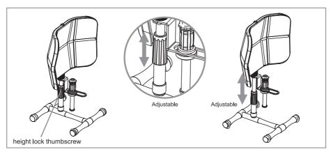
Loosen the stand height lock thumbscrew on mic screen stand with thread(C), you can vertical adjust the position of microphone screen(A) by your own willing. Until mic screen in the proper position, then you can fix the stand height lock thumbscrew.
