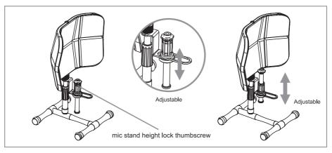
Loosen the mic stand height lock thumbscrew on extension mic stand with thread(D), you can vertical adjust the mic height by your own willing. Until microphone in the proper position, then you can fix the mic stand height lock thumbscrew.
