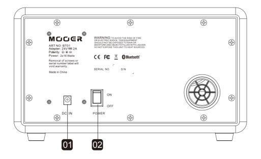
**DCIN:** Connect to a 24V DC power source,  $\oplus - \odot - \odot$ , 2000mA (2A)
