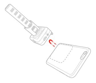
3. Make sure that you position the microphone outside the camera shooting area to avoid the acoustic tube becoming visible in the image frame.
