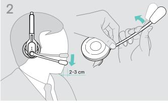
▶ Bend the microphone boom so that the microphone is about O.8" (2 cm) from the corner of your mouth.
