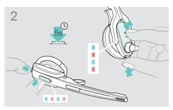
Simultaneously press and hold the Link button and the Audio button for 5 seconds.
