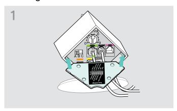
${igle}$  Replace the cover to the rear of the base station.
