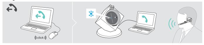
> Start the call using your softphone, the audio signal is automatically transmitted to the headset.
