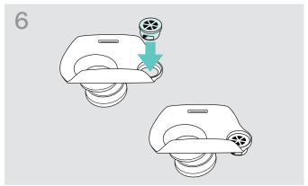
▶ Re-mount ear hook interface – if required – by pushing it in from the backside of the adapter.
