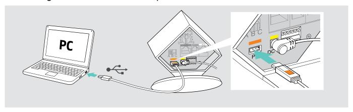
Connect the USB cable to the PC socket (marked orange) on the base station and to a USB socket of your computer. The operating system detects the USB audio device and installs the necessary drivers.
