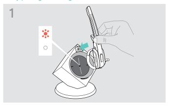
The Link LED on the base station is off (headset is disconnected) or lights up red (no headset paired).
