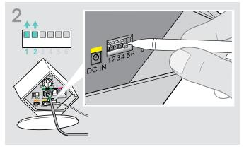
Use a pointed object (e.g. a ball pen) to set the DIP switches 1 and 2 to the position shown.
