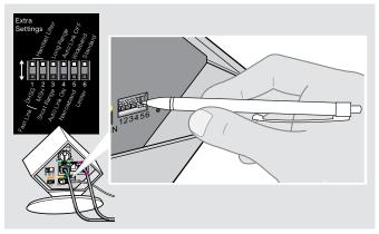
Use a pointed object (e.g. a ball pen) to set the DIP switches to the desired position.
