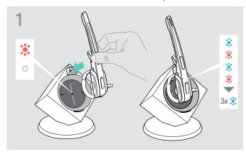
▶ Place the master headset into the base station. The Headset LED alternately flashes blue/red until a link to the base station is established. The Headset LED flashes blue 3 times.
