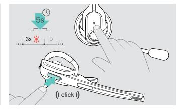
Press and hold the Link button for 5 seconds to switch off the headset immediately.
