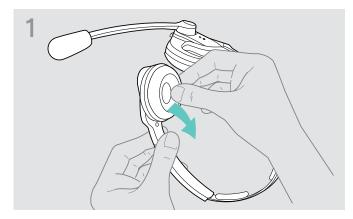
○ Carefully remove the ear pad from the ear cup where the battery compartment is located.
