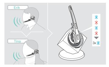
▶ Place the headset to be used into the magnetic holder of the base station.
