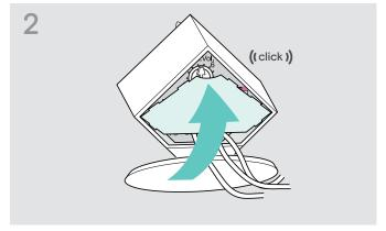
▷ Tilt the cover upwards until it locks into place with an audible click.
