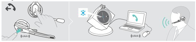
Press the Link button on the headset to establish a link between base station and headset. If the "Auto Audio" function is activated, this step is not necessary (see page 22). Start the call using your softphone.
