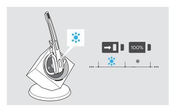
The Headset LED lights up blue and the rechargeable battery is being charged. The Charge status LED on the base station indicates the charge status.
