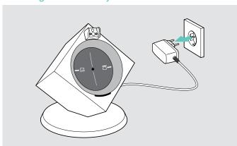
Disconnect the base station from the mains power supply.
