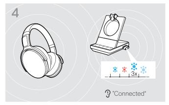
Once the Bluetooth devices are paired, the LED flashes 3 times blue and then lights up in a constant dim blue.
