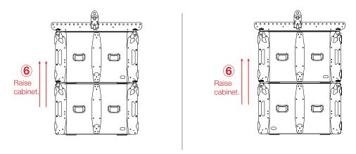
In the same way now, we could add a third enclosure at the bottom. For both configurations, the assembly of AERO-20A, below them is similar:
