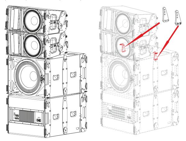
The AX-118S20 accessory, as shown in the figures below, allows to assign an angle for a group of stacked AERO-20A. The central hole corresponds to 0  $^{\circ}$ , while the top hole to -3 $^{\circ}$ , and the bottom hole to + 3 $^{\circ}$ . In summary, the steps will be:
