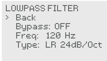
Figure 19. Low-pass Filter adjustment.
