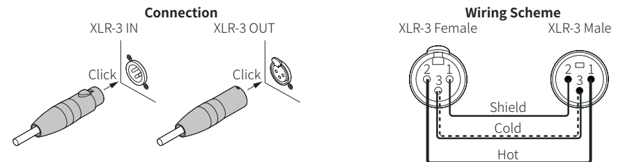
Figure 7. XLR-3 plug-in and cable connection.
