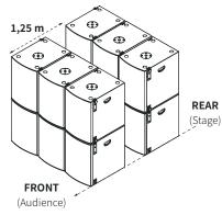
Figure 55. S12 PRO end-fire subwoofer setups Notice the distance is taken from grille to grille.
