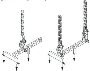
Figure 13. Suspension of the M-F3A BF bumper frame using one or two points.
