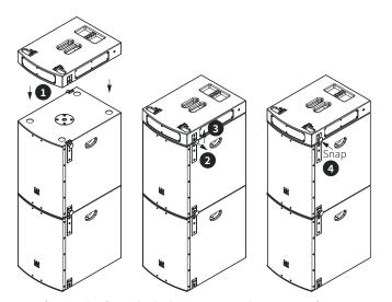
$\textbf{Figure 10.} \ \textbf{Subwoofer ground stack with M-F3A S12 PRO SFi and M-F3A S15 PRO SFi frames.}$
