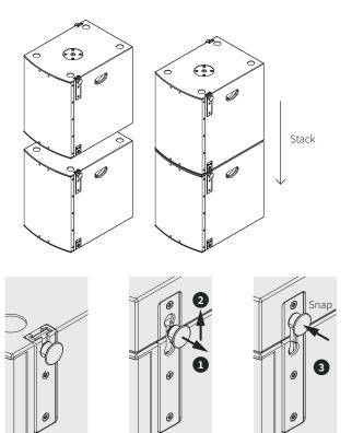
$\textbf{Figure 7.} \ \, \text{Linking system for stacks in S12 PRO and S15 PRO subwoofers}.$
