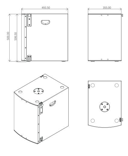
Figure 57. S12 PRO views and dimensions. Annotations given in millimeters.
