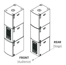
Figure 54. Some configurations for Cardioid setups.
