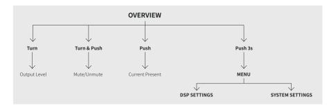
Figure 19. DSP firmware functions and menus.
