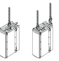
$\textbf{Figure 15.} \ \textbf{Suspension of the M-F3A FS BF bumper frame using one or two points}.$
