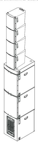
Figure 47. Ground Stack with LF Cardioid Pattern.
