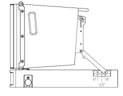
Figure 11. M-F3A S12 PRO SFi and M-F3A S15 PRO SFi rear holes for angle definition.
