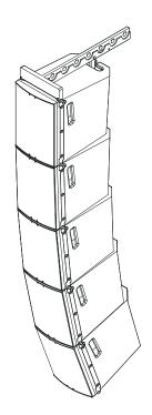
Figure 45. Stand-alone Flown System with 5 units.
