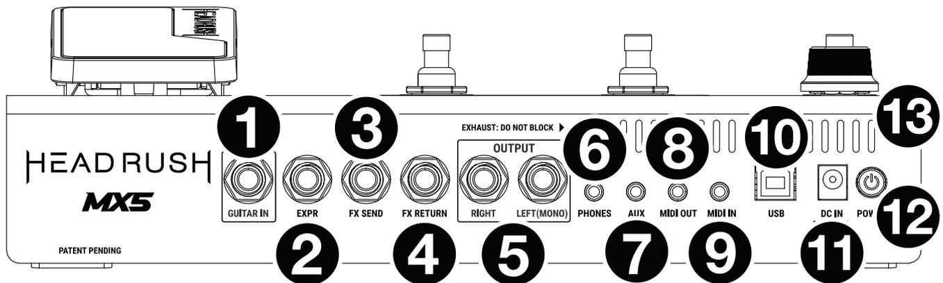
1. **Guitar Input** (1/4"/6.35 mm, mono): Connect your guitar to this input using a standard instrument cable.
