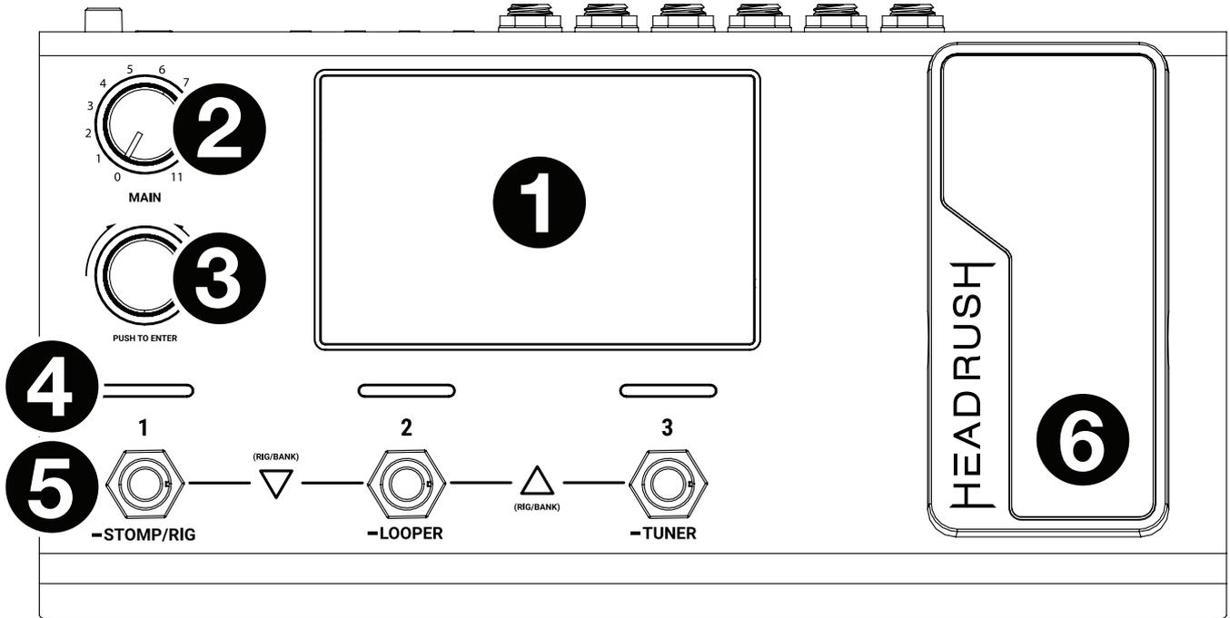
1. **Display:** This full-color multi-touch display shows information relevant to HeadRush MX5's current operation. Touch the display (and use the hardware controls) to control the interface. See [Operation](#) to learn how it works.
