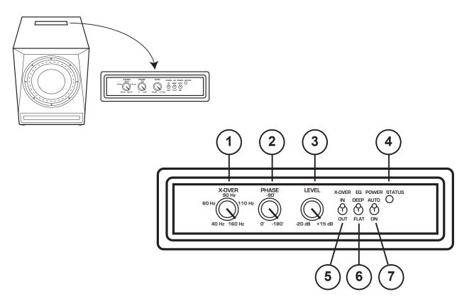
The configuration controls on the Airmotiv RS13 and RS11 Reference Subwoofers are located under a tinted plastic cover located near the rear of the top panel. The cover is attached magnetically - simply lift to remove it and access the controls.
