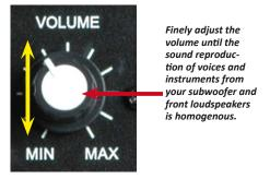
If you can clearly hear the subwoofer, turn down the volume at this point until the sound reproduction of the subwoofer no longer clearly stands out from that of the right and left loudspeakers.
