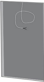
Fig. 3. Drywall Cutout with Speaker Cable
