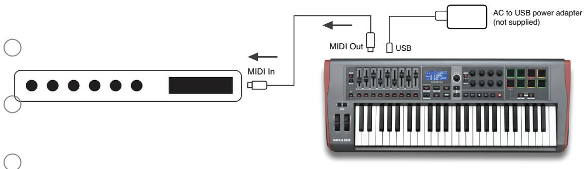
You can also use Impulse to directly control other MIDI-compatible hardware, such as sound modules, FX processors, and so on. To do so, use the standard MIDI ports on the Impulse rear panel and standard 5-pin DIN MIDI cables. As there is no computer to supply Impulse with DC power, you will need to use a separate AC-to-DC adapter designed for USB-powered devices. This is the arrangement you might want to employ in live performance, for example, to avoid the need for an on-stage computer.
