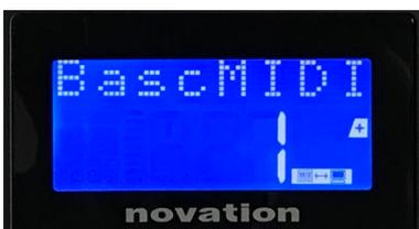
While in HUI mode, a connection icon will appear on the screen, and the Mixer / Plugin buttons will illuminate.
