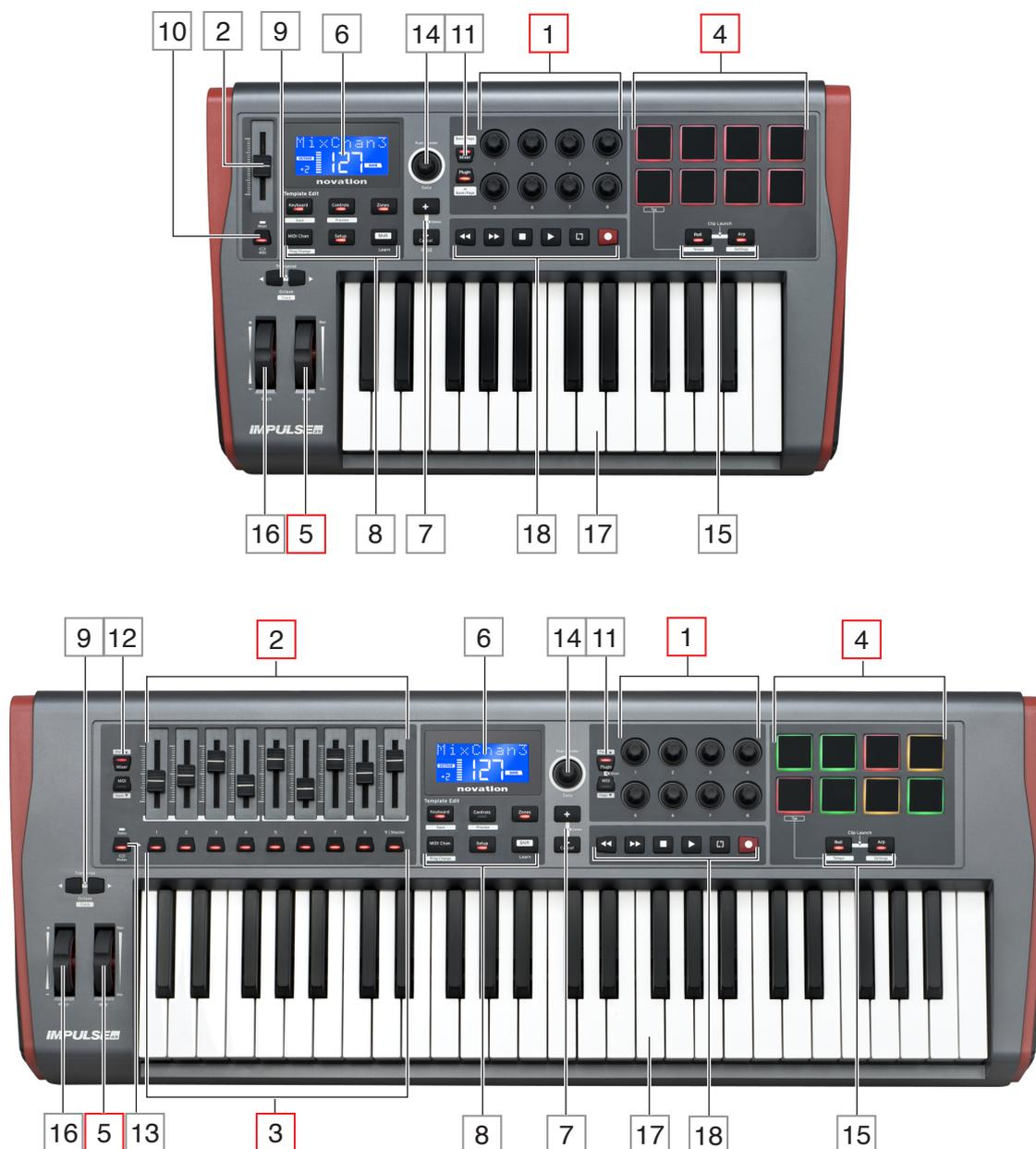
Each of Impulse's controls is either *assignable* or *non-assignable*. Assignable controls are 'free' – their function will vary according to which plug-in, DAW mixer or additional piece of MIDI hardware is being controlled. Their assignment to a particular parameter of the Thing being controlled will either be made manually by you. Non-assignable controls are 'fixed' – their function will generally always be the same regardless of what sort of setup you are using
