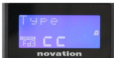
Operating any assignable control – e.g., faders 1-9\*, buttons 1-9\*, encoders 1-8 or the drum pads – makes the display show parameter for that control. The selected control number is displayed, for example **Fd3** (Fader 3) or **Bt5** (Button 5).
