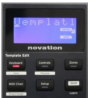
The character to be edited is the one with the flashing cursor; use the Data knob [14] to alter the character, and the **+ / -** buttons [7] to shift the character position. When you have finished editing the name, press **Enter**, and a **SaveTempl?** (Save Template?) confirmation screen appears. If you are happy that you are saving the altered name to the
