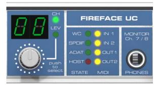
**Phones** is a low impedance line output of highest quality. It provides a sufficient and undistorted volume even when used with headphones.
