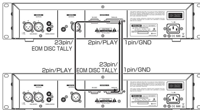
By connecting three or more CD-6010 units in sequence (**CONTROL I/O PARALLEL** "2 PLAY" to **CONTROL I/O PARALLEL** "EOM DISC TALLY") as shown below, automatic playback of one unit after the other is possible.
