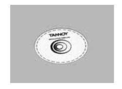
Cut out the hole in the ceiling using a circular saw or pad saw, then slide the C-ring into the ceiling, aligning it over the cut-out hole).
